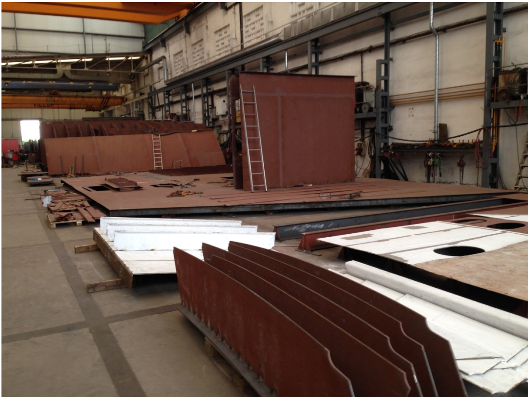
BL 14 - Tween Dk. with cofferdam between Clean SW Lab & GW tank – BL06 in background
