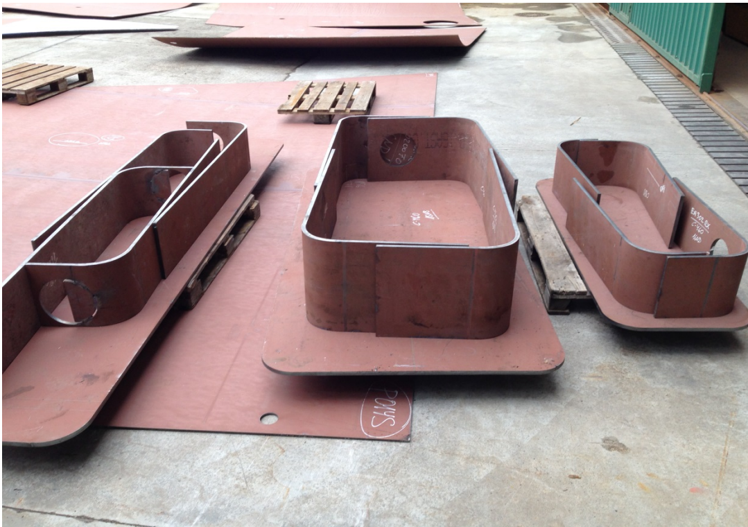
Casings for EM 302 & SBP 300 ready for installment in BL 05
