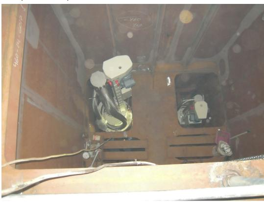
Hatch from Lab 26 to drop keel trunk
