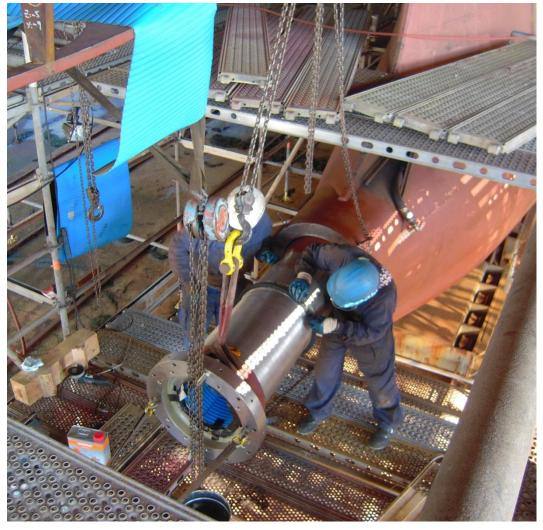
Rudder stock tube installed
