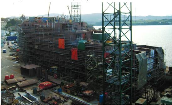
44 blocks placed and assembled on slipway by 31.10.15
