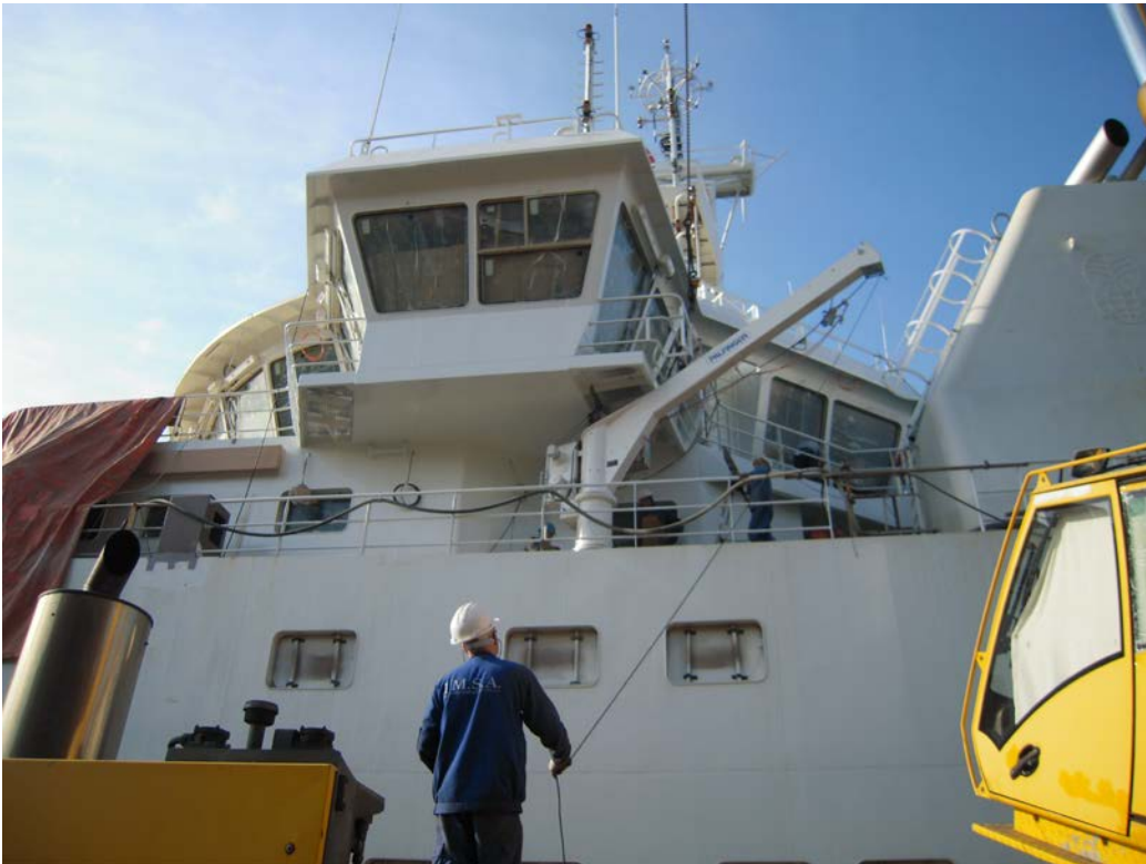
Crane for life rafts installed
